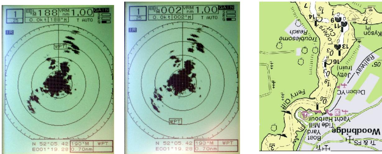
Fig. 1. Radar screen from *Ragged Robin* in Tidemill YH looking south towards Loder's Cut. Left: Compass input. Waypoint marking Loder's Cut shown in correct place ahead (S) of vessel. Middle: GPS input only. Loder's waypoint incorrectly located behind (N) of vessel because the radar has interpreted the GPS track (002 deg) as the ship's heading (see top of screen). Right: inverted chart showing upper part of radar picture location.
