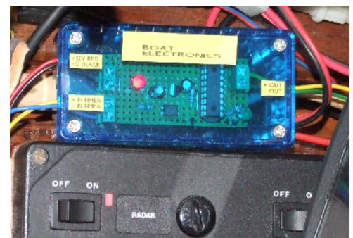
Fig. 2. Compass-radar (NMEA) interface in *Ragged Robin*.
